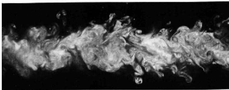
174. Turbulent wake of a cylinder. A sheet of laser light slices through the wake of a circular cylinder at a Reynolds number of 1730. Oil fog shows the instantaneous flow pattern, covering 40 diameters centered 50 diameters downstream. Photograph by R. F. Fales
