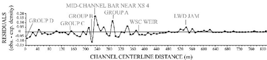
Figure 4. Tracer density residuals along the channel centreline (observed density minus density predicted from gamma model). The distribution highlights the influence of morphological constraints.
