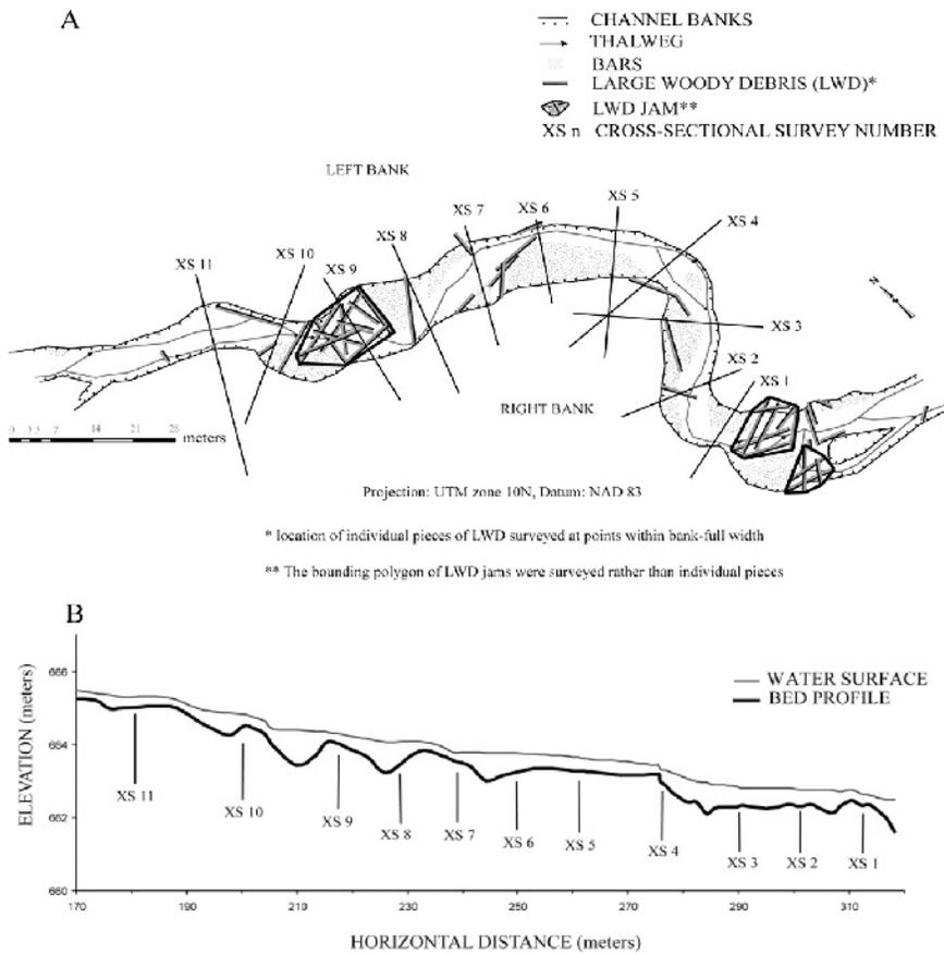
Figure 3. A. Planimetric study area map with the location of cross-sectional bed elevation surveys 1–11 labelled. B. Thalweg longitudinal profile. The location of cross-sectional surveys has been added for reference.
