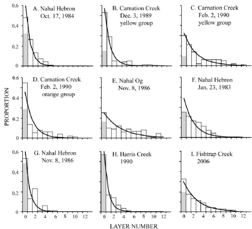
Figure 5. A-H. Depth distribution of all moved particles. Source: Hassan and Church (1994). (I) Fishtrap Creek depth distribution of moved particles from all groups. Layers represent scaled intervals of burial depth equal to the median grain size of the surface for each river. Gray areas represent particles exposed on the surface.
