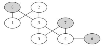
**SOLUTION:** We'd use the edges: (0,3),(3,4),(4,7),(4,6) to produce the minimum Steiner Tree. Note that this is a tree but **not** a spanning tree!
