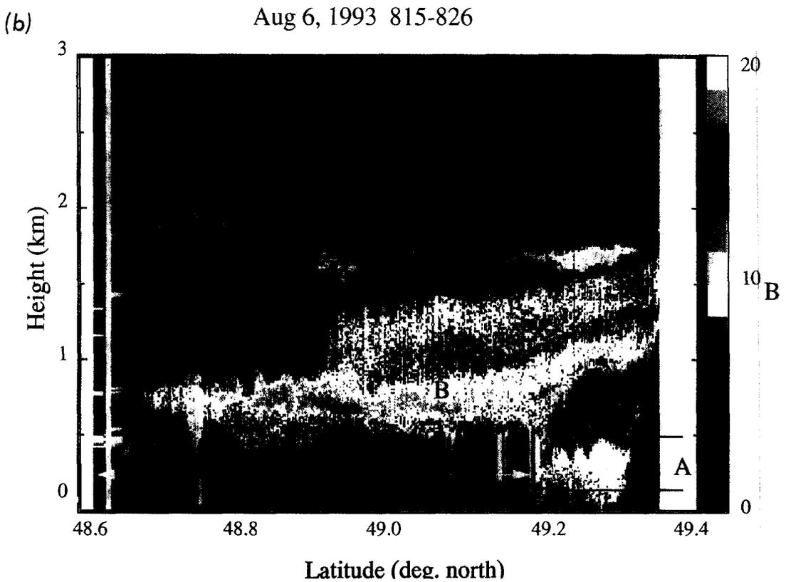
Fig. 3. Aircraft lidar north-south transect showing aerosol backscatter for (a) 5 August, 1355-1406 PST and (b) 6 August, 0815-0826 PST. Prominent features discussed in the text are labelled. The colour scale represents the ratio of total backscatter to that of clear air (Rayleigh).
