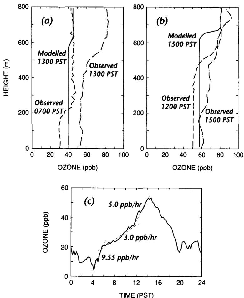
Fig. 8. The modelled effect of vertical down-mixing on boundary layer ozone concentrations at Harris Road based on initial profiles at (a) 0700 PST and (b) 1200 PST. Ground-level ozone concentration observed at Harris Road with observed rates of change are shown in (c).
