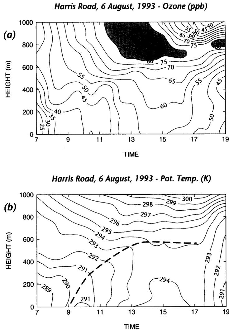
Fig. 6. Time-height plots showing isopleths of (a) ozone concentration and (b) potential temperature based on tethered balloon profiles from Harris Road for 6 August 1993. In (b) the growing mixed layer is denoted by a dashed line.
