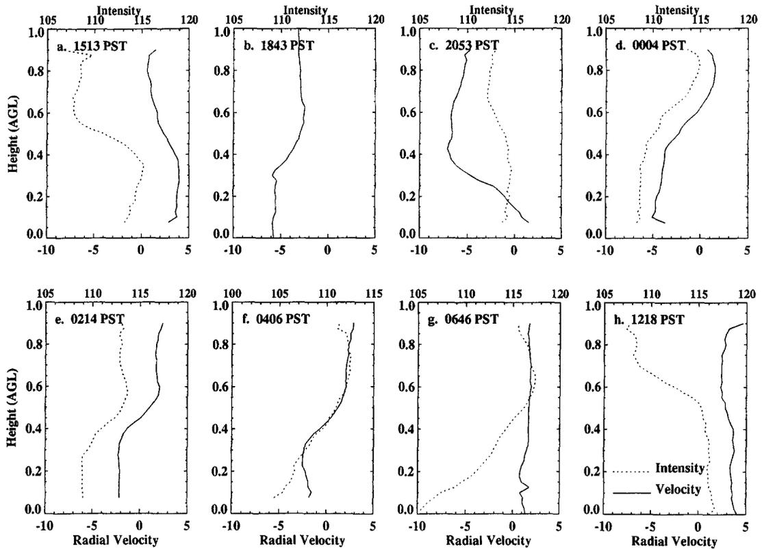
Fig. 5. Profiles of radial velocity (solid lines) and backscattered signal intensity (dashed lines) averaged over 1 km. Averages were derived from the vertical cross sections shown in Fig. 4 for 4/5 August 1993. The lower x-axis gives the radial velocity scale ( $\text{m s}^{-1}$ ), and the upper x-axis, intensity (arbitrary dB units).
