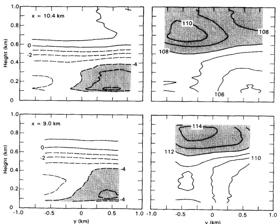
Fig. 6. Cross-flow vertical cross sections from the 0004 PST high-resolution lidar volume scans on 4/5 August 1993, shown schematically in Fig. 2 as line AB. The top two plots show contours of  $u_r$  (left,  $\text{m s}^{-1}$ ) and backscattered signal intensity (right, dB) 10.4 km from the lidar. The bottom two plots show similar contours from the same volume, but at a distance of 9 km from the lidar. Radial velocities  $> 4 \text{ m s}^{-1}$  and areas of highest backscatter are shaded.
