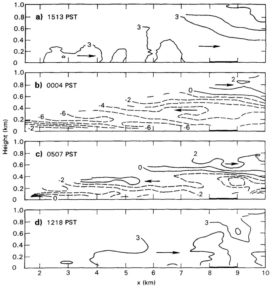
Fig. 4. Vertical cross sections of lidar radial velocities for 4/5 August 1993 along the 28° azimuth, line OP in Fig. 2. The lidar is at (0,0). Positive values (solid contours) represent flow away from the lidar (upvalley), and negative values (dashed contours), flow toward the lidar (downvalley). The bold line from 8 to 9 km (along the x-axis) shows the region where data were averaged for the profiles in Fig. 5.
