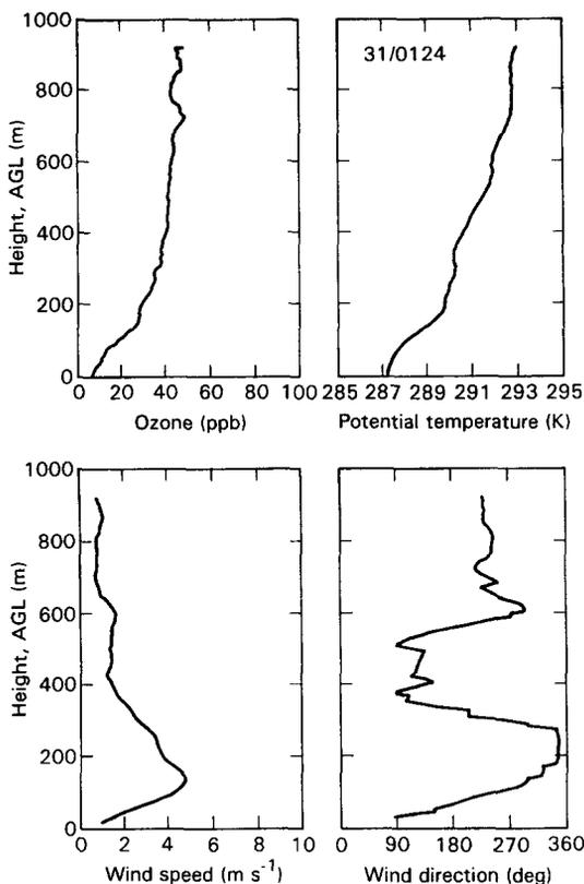
Fig. 7. Profiles of ozone, potential temperature, wind speed, and wind direction from a tethered sonde launched from a site on Little Goose Island, in Pitt Lake at 0124 PST, on 31 August 1994.
