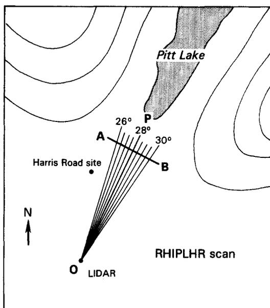
Fig. 2. Diagram of the high-resolution volume scan performed regularly by the ETL Doppler lidar during the Pacific 93 study. Each ray toward Pitt Lake represents a vertical slice scan. Vertical, along-the-beam cross sections of flow coming out of Pitt Lake valley (OP) and beam-perpendicular vertical cross sections (AB) were used for analyzing lidar volume scans.
