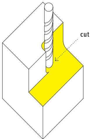
It is possible to create objects with tighter tolerances and better finishes using subtractive manufacturing. When it comes to precision for common functional features such as flat surfaces, drilled and tapped holes, counter sinks, and counter parts, subtractive processes generally achieve results with maximum repeatability and dimensional accuracy. Subtractive fabrication can also apply to 2D objects cut from flat stock.
