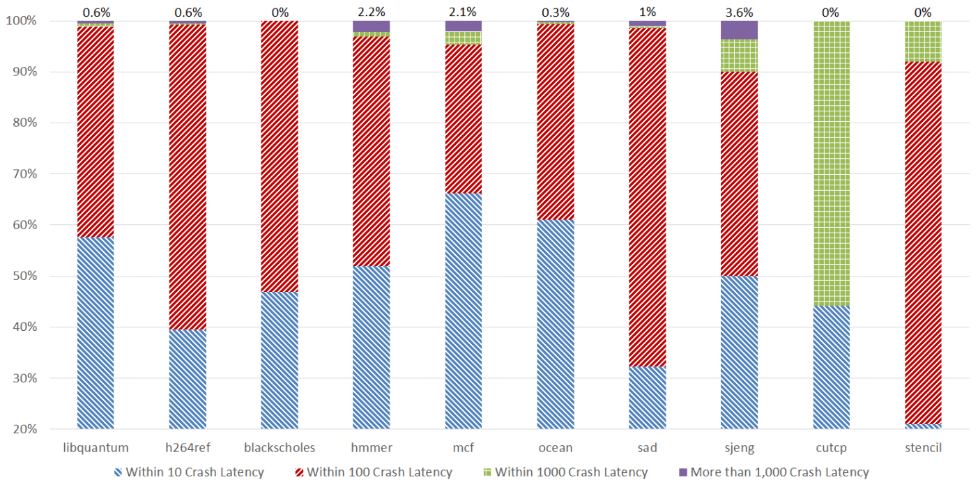
Fig. 3: Latency Distribution of Crash-Causing Errors in Programs: The purple bars represent the LLCs as they have a crash latency of more than 1000 instructions. The number shown at the top of each bar shows the percentage of crashes that resulted in LLCs. The error bars for LLCs range from 0%(cutcp) to 1.85%(sjeng).
