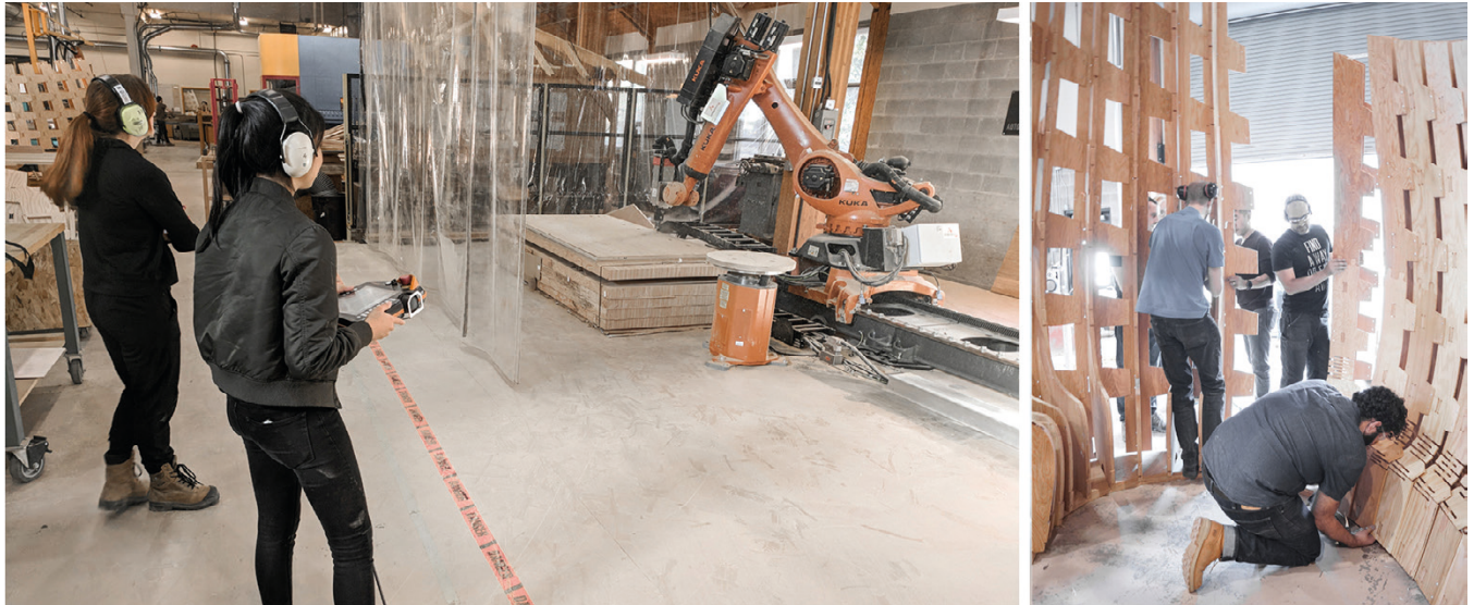
5 Robotic fabrication and modular assembly process. Each piece was cut in a 5-axis CNC process using an extended 7-axis robotic setup. Afterwards, the elements were assembled into 5 separate modules small enough to be transported across campus. The assembly took place in the workshop under controlled conditions. The modules were then assembled on site into the final demonstrator.
