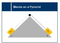
Exploration of free body diagrams, two body acceleration, and newton's laws through the system of two blocks resting on a pyramid and attached by a pulley.
