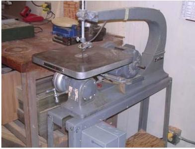
The scroll saw uses a tensioned reciprocating blade to cut. The material is slid over a table similar to that of the band saw. The scroll saw is usually used without a fence. The reciprocation speed can be varied by altering the belt and pulley configuration and the table can be tilted. Because of the narrow blades available and the amount of control possible over blade tension and speed, this machine is good for making fine curvy cuts through thin material.
