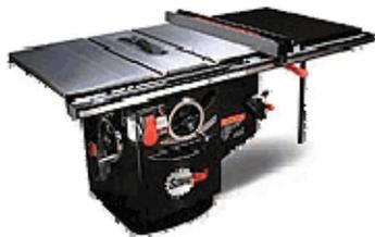
The table saw is often the centre of the shop in terms of both layout and use. It is the largest machine in many shops, requiring the most infeed and outfeed space and has a versatility that allows it to be used for several stages of construction. It can do most basic cutting jobs as well as a good deal of refined milling and joinery work. With a sharp blade it will give a straight, relatively clean cut.
