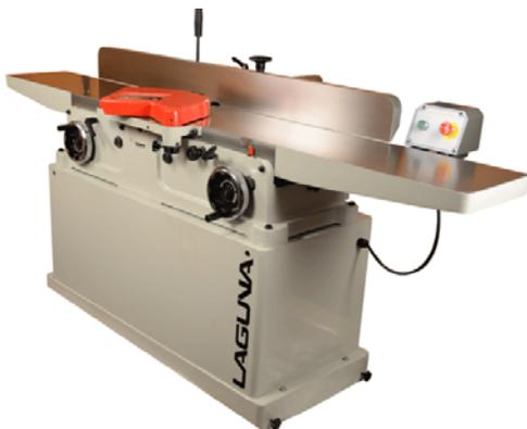
The jointer removes material from underneath the board. Varying the difference between the planes of 2 parallel tables – the “infeed” and the “outfeed” - controls how much material is removed. By keeping the cut surface pressed to the outfeed table as the wood is fed over the cutter, a straight, flat surface can be obtained.
