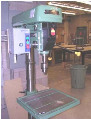
There are 2 drill presses in the shop. They are used to drill holes in material at controlled angles and depth. Because of the bed or table to which material can be clamped, either directly or by way of a jig, multiple identical holes can be drilled.
