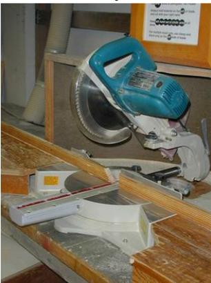
this piece is too small to be safely held, you should be using the table saw with a sled. (See "Table Saws") If using a clamped stop block for multiple cuts, it is particularly important that the piece between the blade and the stop block be securely held during the cut, to avoid kickback.
