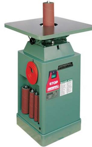
When changing drums, note that the bolt is reverse threaded. Also remember to select a red collar insert that fits the size of drum being used.
