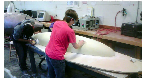
Above, team members sand the plug for the most recent competition hull. The plug was CNC cut from foam and coated in a durable plastic compound. This was used to make a fiberglass mold for the hull.
