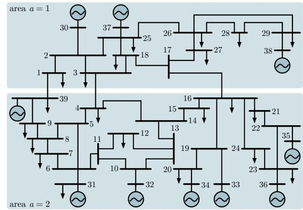
Fig. 3: One-line diagram for the New England test system.
