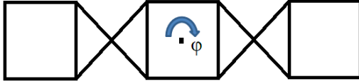
Figure 2: Schematic illustration of 1D block (square)-spring (diagonal lines) mechanical model that can support rotational waves. \Phi refers to the rotational degree of freedom of the blocks.
