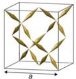
Cellular structure with pentamode behavior, created by optical lithography
