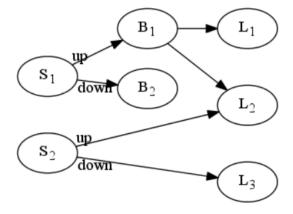
SOLUTION: A working configuration would be  $S_1$  is up (which powers  $L_1$  and  $L_2$ ) and  $S_2$  is down (this powers  $L_3$ ).
