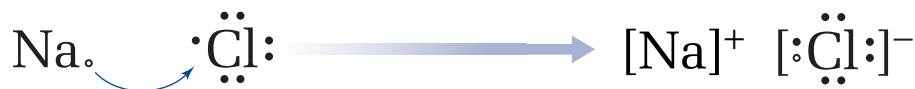
Figure 3.10 These Lewis structures show the formation of a bond between a sodium atom and a chlorine atom.
