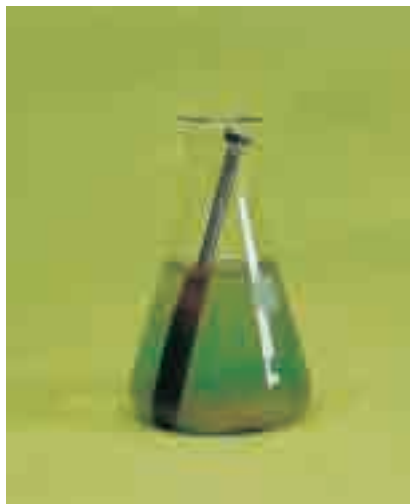
Figure 4.13 When an iron nail is placed in a solution of copper(II) sulfate, a single displacement reaction takes place.
