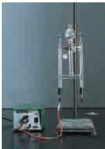
Figure 4.8 As electricity passes through the water, it decomposes to hydrogen and oxygen gas.
