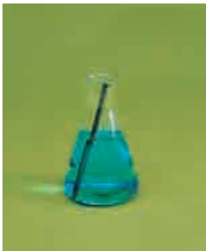
Figure 4.13 When an iron nail is placed in a solution of copper(II) sulfate, a single displacement reaction takes place.
