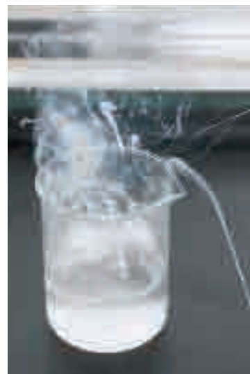
Figure 4.12 Lithium metal reacts violently with water in a single displacement reaction. Lithium must be stored under kerosene or oil to avoid reaction with atmospheric moisture, or oxygen.
