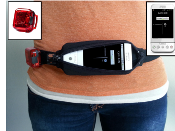
Example of an accelerometer that feeds data to a mobile device (Donaire-Gonzalez, D., et al., 2013)
