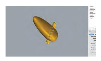
After many attempts using Curve Network, arms were created using the contours as a template instead for manipulating primitive shapes. A cylinder-like shape and Split tool were used to create voids and surfaces of palm. These surfaces were scaled and manipulated with control points and blended back together with BlendSrf. Complete arm was further stretched and pulled to scale using control points.
