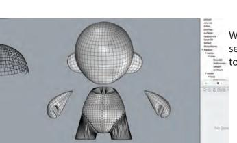
Water-tight pieces were converted to meshes and kept seperate for ease of manufacture. Pieces were put back together for export to KeyShot.
