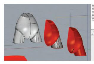
Once the solid body was created, a leg wascreated by lofting between two contours. Foot was filleted and leg was attached using boolean difference followed by blend surface. The body was split and the body/leg was mirrored to complete this step.
