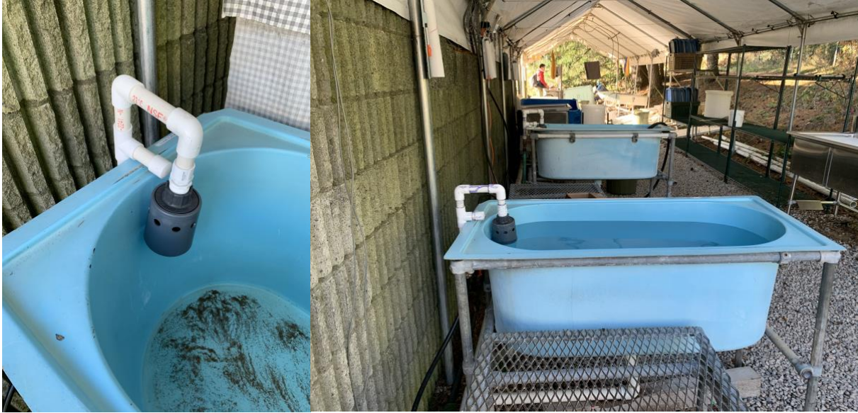
Figure 7. (Left) Hudson valve set up close up. (Right) Hudson valve installed on all four tanks. Tank 1 shows the maximum water level in the tank.
