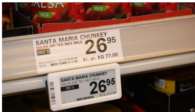
Figure 4. An electronic shelf-label. Image source: https://www.eink.com/electronic-shelf-label.html?type=application&id=5
