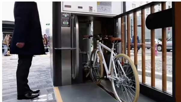
Fig. 5. GIKEN LTD; Automated Parking Facility ECO Cycle. 2019
