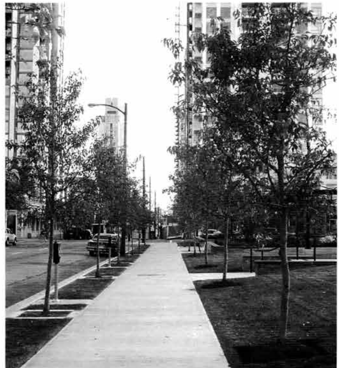
Figure 2.1.5. Trees in easy (right) and difficult (left) places will never grow at the same rate and already show differences in growth after just a few years. This designer added grates around the street-side trees, making an already difficult place even more difficult for the tree.
