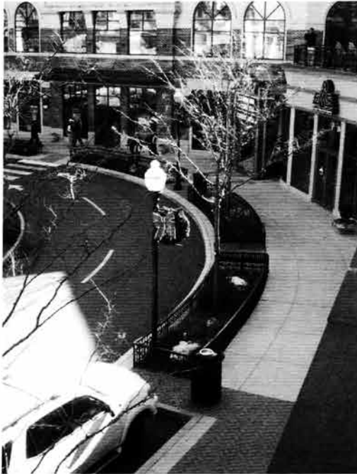
Figure 2.2.3. Long planting spaces allow the largest open soil space while accommodating other urban functions.
