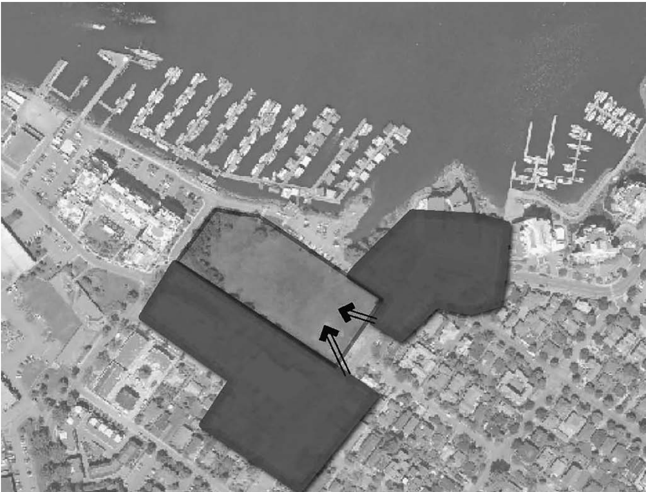
Figure 5 The stormwater outflows of these two catchment areas adjacent to Fishermen's Wharf Park are now treated by the large rain garden within the park.
