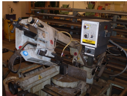
Step 2: Measure to 6" and cut on band saw
