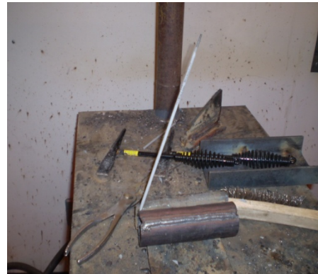
Step 5: watch out for electrode stick.
