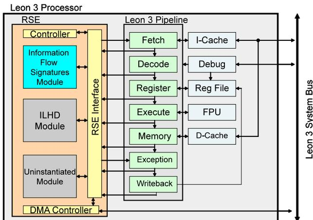
Figure 2: The Leon 3 processor with the RSE Interface
