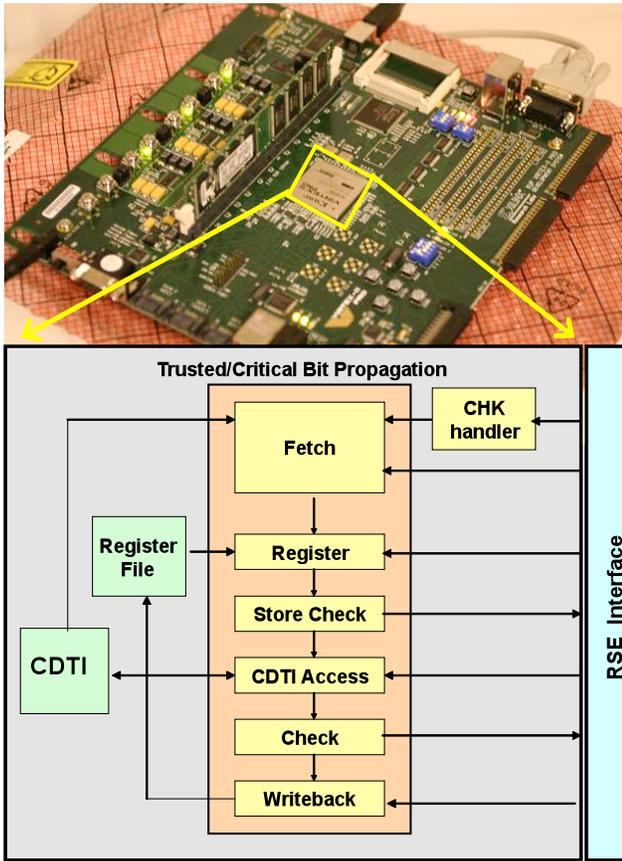
**Figure 3: Diagram of the Information Flow Signature Checking Module and Photo of the FPGA Board**
