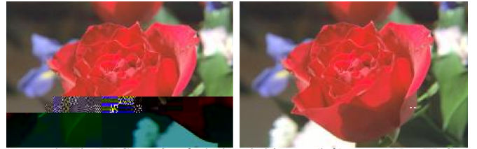
Figure 1: The EDC causing fault decoded image (left) versus Non-EDC causing fault decoded image (right) from the JPEG decoder
