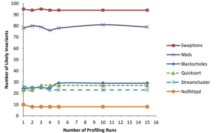
Fig. 5: Number of invariants generated from varying numbers of profiling runs for six benchmark applications
