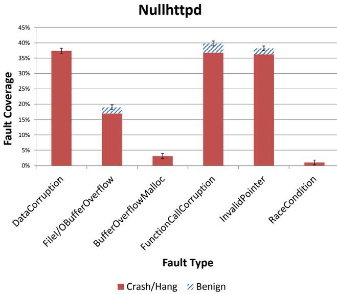
Fig. 10: Proportion of 1000 faulty Nullhttpd runs that violate at least one invariant
