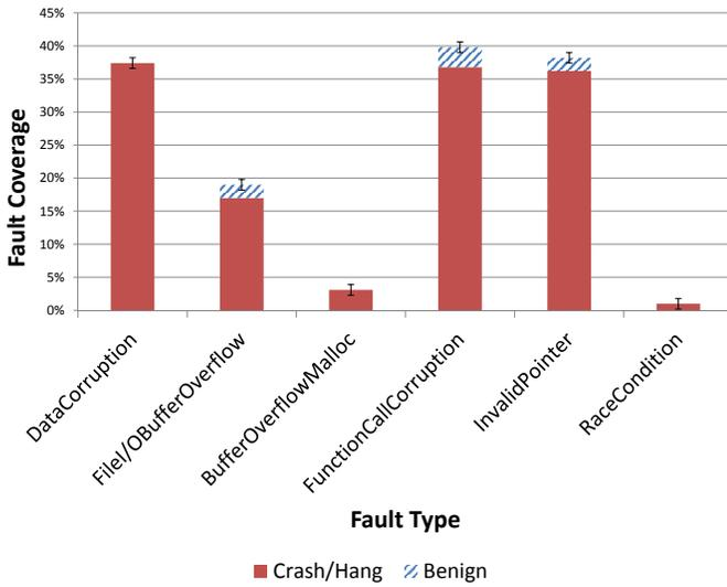
Fig. 10: Proportion of 1000 faulty Nullhttpd runs that violate at least one invariant
