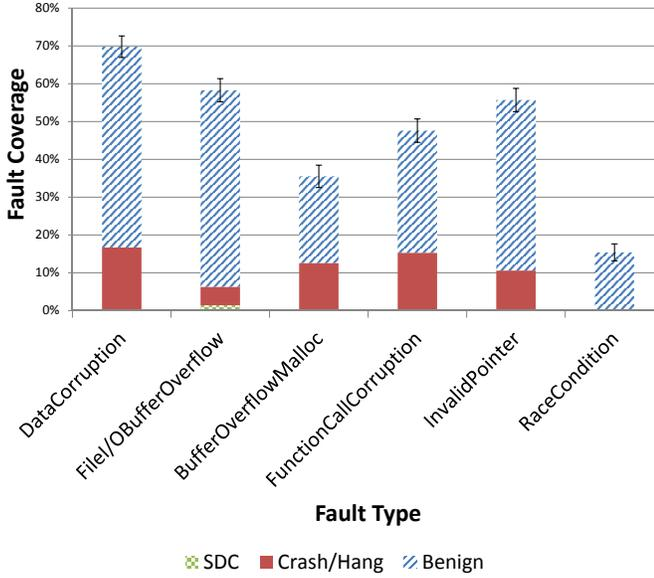
Fig. 9: Proportion of 1000 faulty Streamcluster runs that violate at least one invariant
