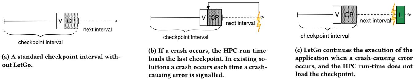
**Figure 1: Illustration of how LetGo changes the behavior of an HPC application that uses checkpointing by continuing the execution when a crash-causing error occurs. Axes indicate time. The labels used for time intervals: CP - checkpoint; V - application acceptance check/verification; L - LetGo framework, lightning bolt: crash-causing error**
