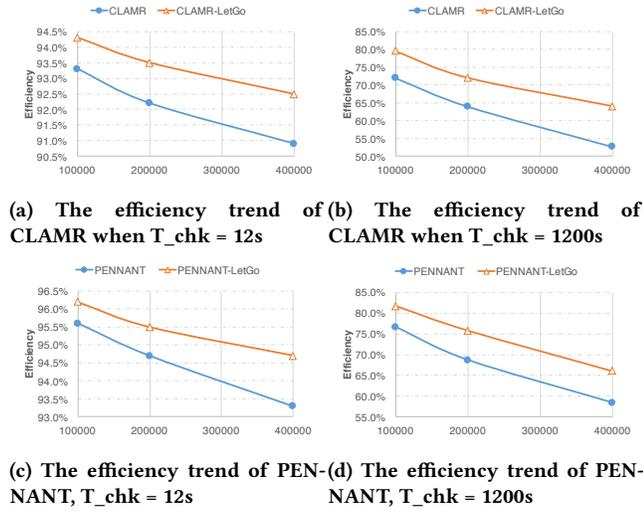
**Figure 8: The trend of the efficiency for the C/R scheme with and without LetGo when the system scales from 100,000 nodes to 200,000 nodes and 400,000 nodes**
