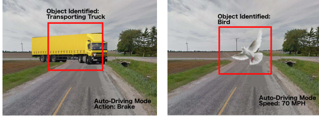
(a) Fault-free execution: A truck is identified by the DNN and brakes are applied (b) SDC: Truck is incorrectly identified as bird and brakes may be not applied
