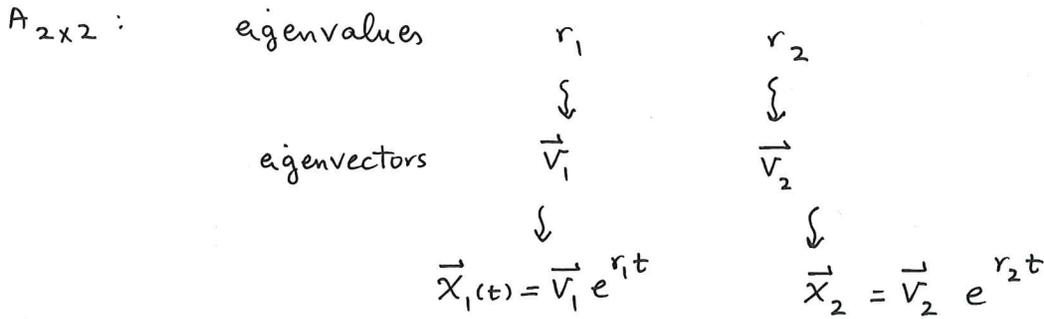
General solution:  $X(t) = c_1 \vec{X}_1(t) + c_2 \vec{X}_2(t)$
