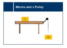
Exploration of free body diagrams, two body acceleration, and Newton's law through the system of two blocks attached through a pulley and one of them resting on a table. acceleration, forces, friction, Newton's laws,
