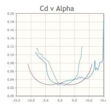
This shows the NACA 0015 having lower drag across the range of 2° to 8° angle of attack. That means this airfoil may result in a plane that is capable of flying faster than the other two airfoils. Since total lift is a function of both Cl and airspeed, and airspeed is squared, while Cl is linear, the lower drag may offer lift advantages over the other two airfoils with higher drag, IF your fuselage and propeller are designed to allow the aircraft to travel at higher speeds.
