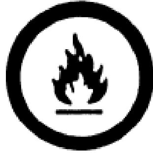
Flammable and Combustible Material
