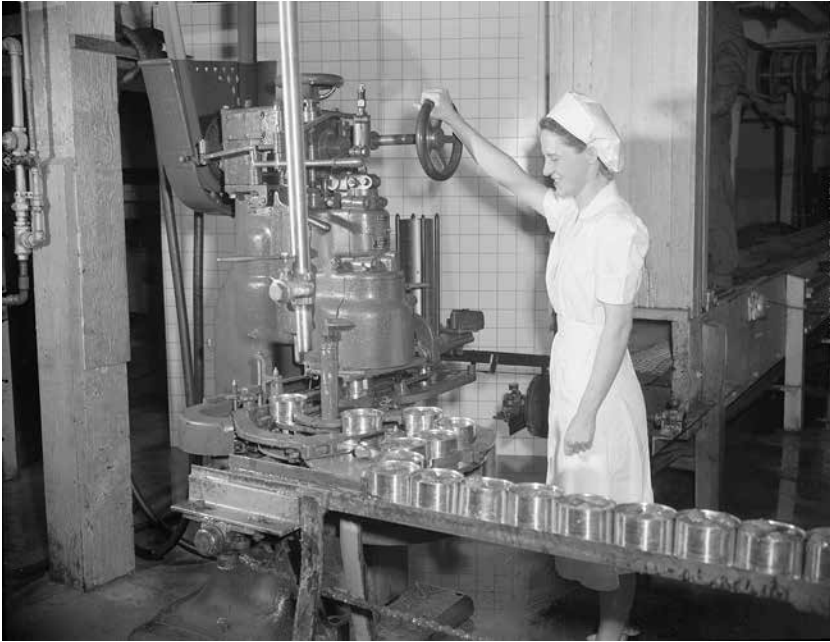
Figure 5. A woman worker operates a semi-automated machine to seal cans of meat at Hedlund's Fancy Sausage Ltd. in Vancouver, ca. 1947. Jack Lindsay, "Woman operating machine to seal cans of Hedlund's Ltd. meat products," ca. 1947, Jack Lindsay Ltd., City of Vancouver Archives, Photographers Fonds, 1184-3554.
